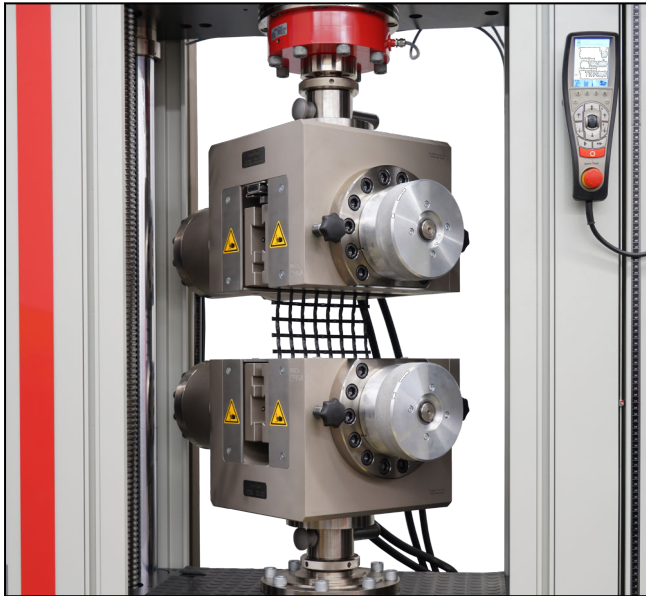
Type 8593 hydraulic grips, Fmax 250 kN
