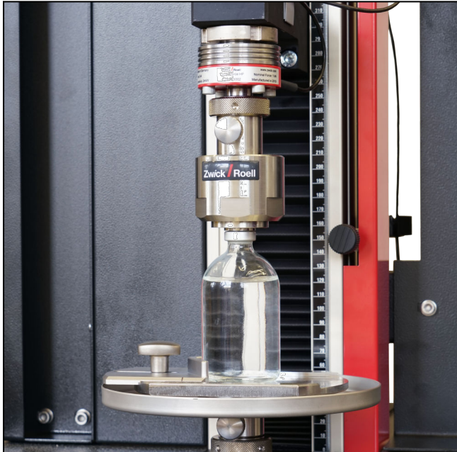
Fixture for determining the residual seal force
