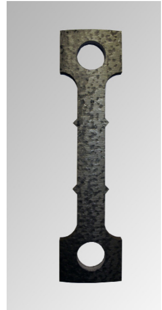
Pipe-segment specimen with collars in parallel length
