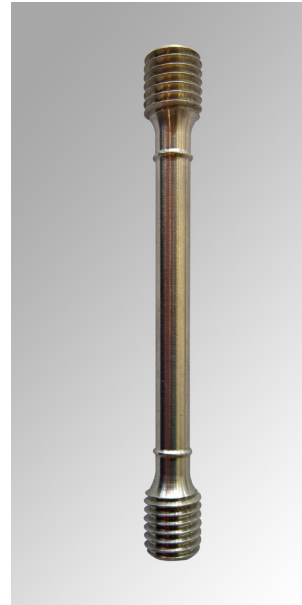
Round specimen with collars in parallel length
